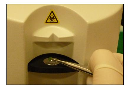
11. Keep track of the osmometer measurements. When the osmolality value changes less than 5 mmol/kg then the value has reached equilibrium. This usually takes about 10-15 minutes, or 4-5 measurement cycles.
